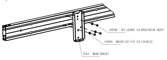
Secure the quick link to the mounting bracket and insert end chain link, secure the arm support channel to the mounting brackets, insert a bolt
