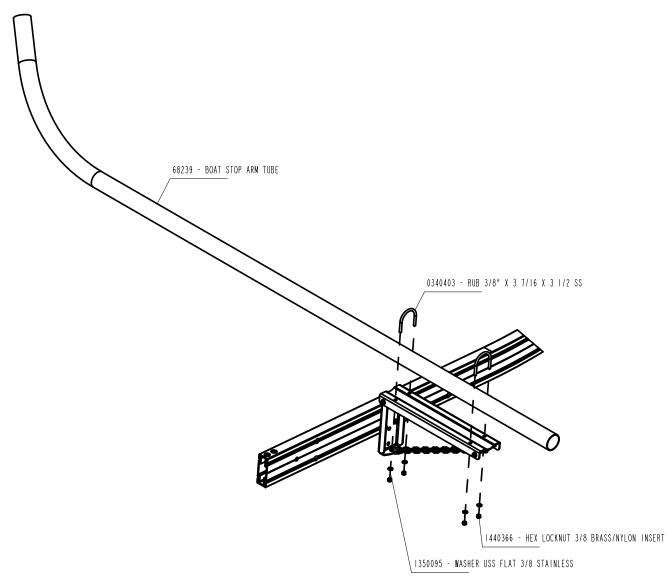
Mount the stop arm tube as shown using the hardware included with the kit. Repeat this process on the other side.
