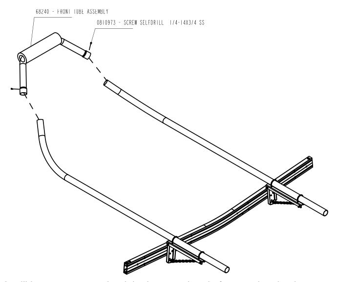
It will be necessary to load the boat on the platform and make the necessary adjustments before finishing the assembly to properly fit it to the boat. Adjust the chain links to ensure that the front tube assembly is just above the bow eye. Make sure all mounting components are in place and center the assembly before tightening the hardware securely.
