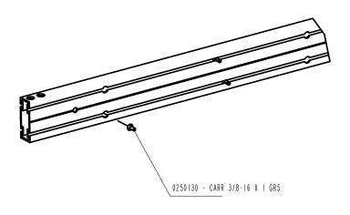
Insert mounting bolts into the slots on the inside of the platform v-frame and slide toward the desired location. One in the top and two in the bottom and slide them toward the center.
