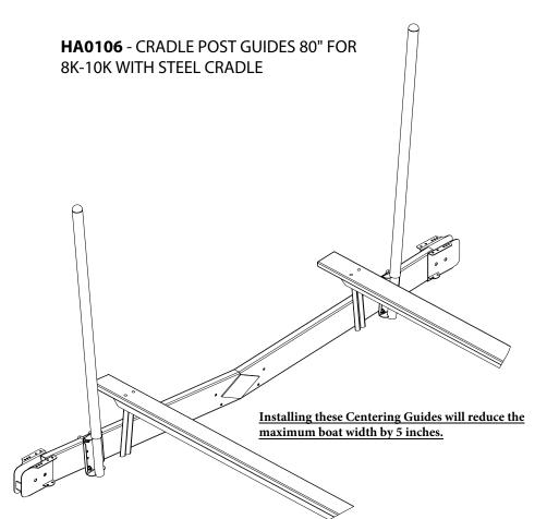
The **HA0106/HA0291** is intended to be used in conjunction with the **HA0107/HA0292** spring loaded post load guides. It is to be mounted on the front platform of the lift and is to be adjusted inward or outward to center your boat as it is loaded onto the lift.
