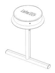
**5)** Bolt the seat pan to the top of the seat post with foot hanger using the four M5x8mm screws from Bag C.
