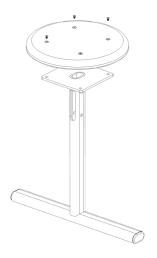
**7)** Bolt the seat rail with ratchet to the seat post with foot hanger using the  $3/8-16 \times 1/2$ " bolts from Bag C.
