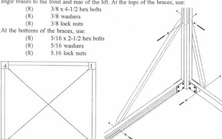
Square the mainframe by measuring its diagonals. The diagonals must be equal. If they are not, adjust the mainframe until they are. Once this is accomplished, tighten all of the bolts except the  $5/16 \times 3$  hex bolts. The cables in the rear cradle will attach to these.
