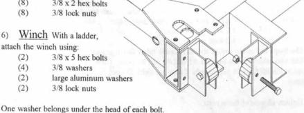
The aluminum washer and the other washer go under the nut on the outside of the lift.
